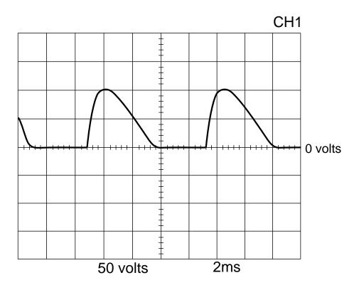
This is the typical DC (+) output voltage waveform generated from a properly operating machine. Note that each vertical division represents 50 volts and that each horizontal division represents 2 milliseconds in time.
